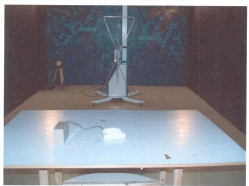
6.2. Photo of Electrostatic Discharge Test
